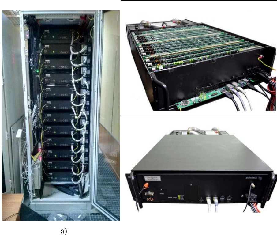
Fig. 5. RCS Nekkar based on advanced computational modules (a – without heatsinks, b – with placed heatsinks)
