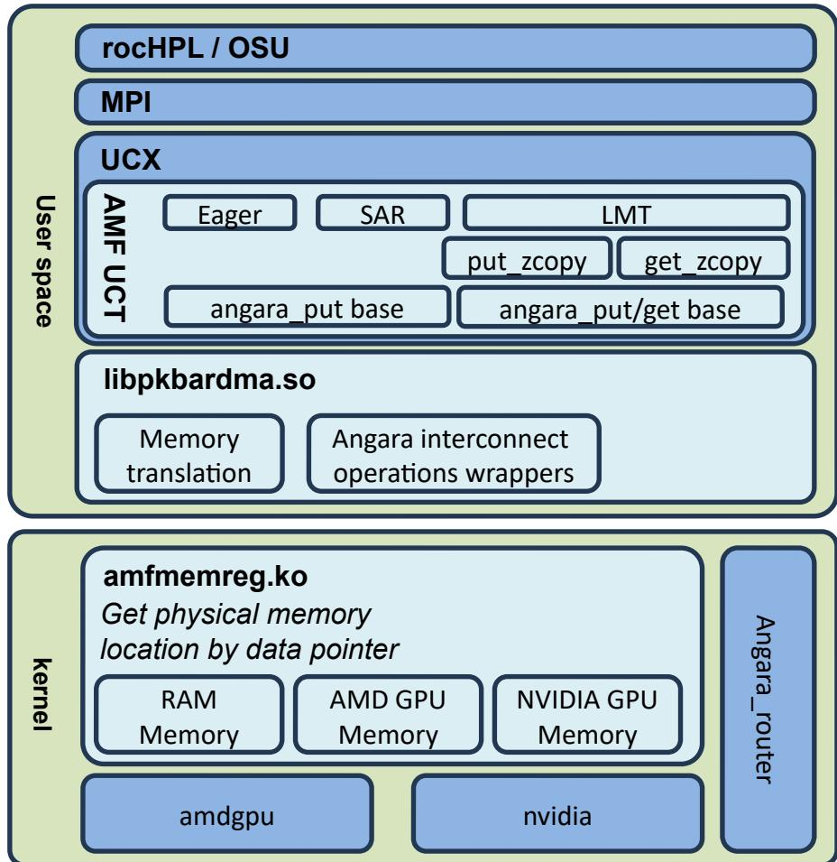
**AMF UCT** – Transport in UCX implementing support for remote GPU or HOST memory reads and writes by extended Angara API.
