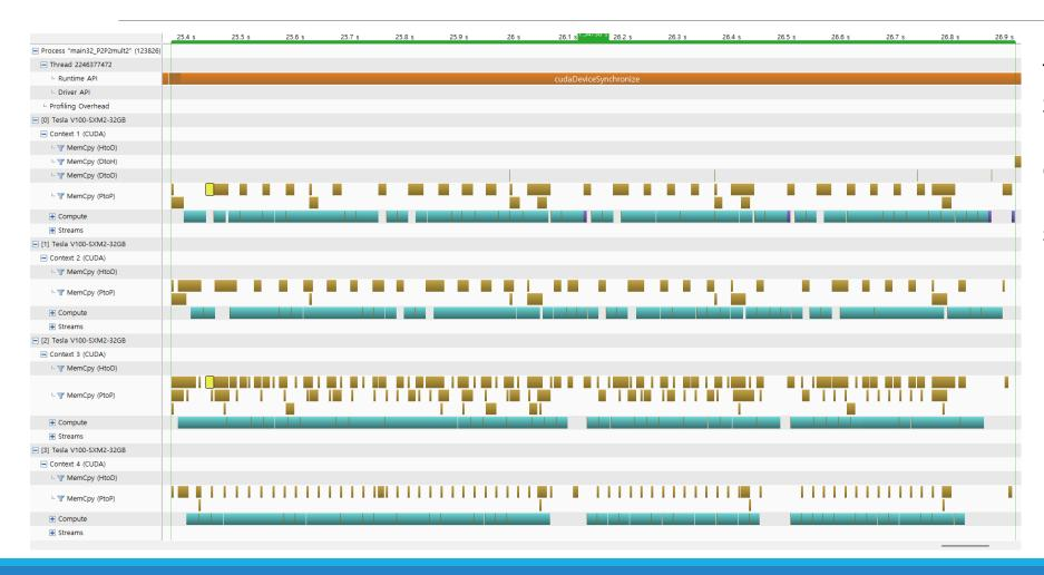
The profile of the Multi-GPU SGEMM operation on IBM POWER 9 server. Number of elements (N = 32768) in a row (column) of matrices, and tile sizes (N<sub>i</sub> = 2048 and 4096). Matrices A, B, and C are stored in devices 1, 2, and 0, respectively.
